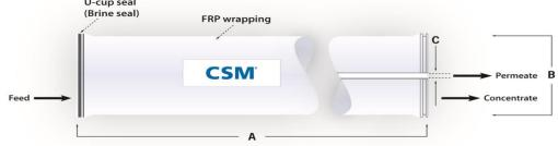
1. Each membrane element supplied with one brine seal, one interconnector (coupler) and four o-rings. 2. All NE8040 elements fit nominal 8.0 inch (203.2 mm) I.D. pressure vessels.
